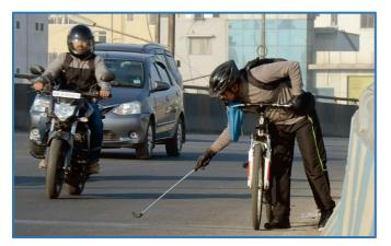
At first, he would pick up the nails by hand, but soon realized that it was a very timeconsuming and ineffective method, so he built a tool to help him on his cleaning runs. He took one of his broken fishing rods and modified it by attaching magnets to one end and making it foldable.
